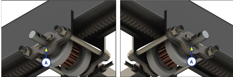
Figure 41. Gear Pack lubrication points - exterior.
