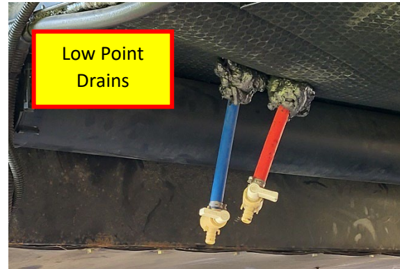
Figure 131. Water system low point drains.
