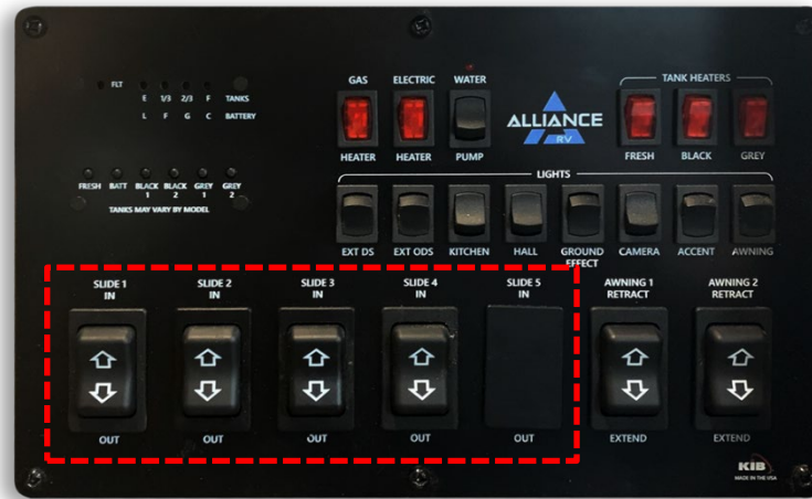
Figure 35. Monitor panel with slide-out controls highlighted.
