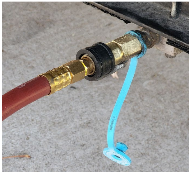
Figure 33. Connected appliance, with flow lever rotated forward to the "on" position.
