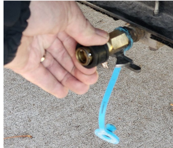
Figure 32. Pushing the retaining ring to accept an appliance connector.
