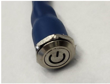
Figure 65. Renogy battery activation cable - power button (switch).
