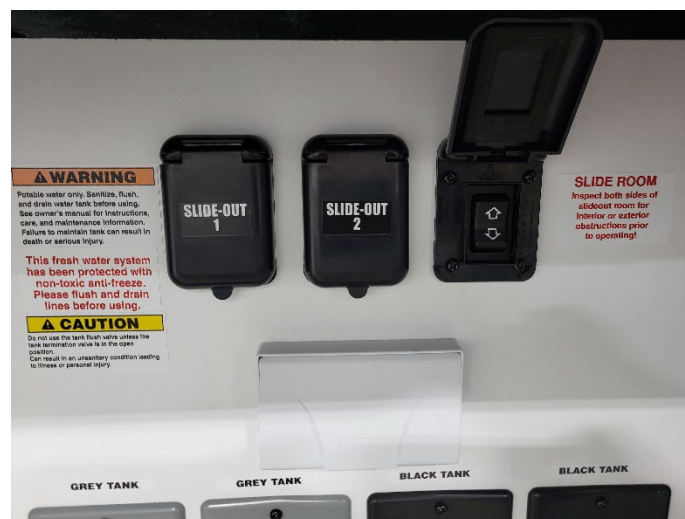
Figure 36. Remote slide controls in the utility bay of the Avenue.
