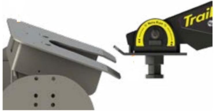
Figure 13. Appropriate vertical position to assure safe kingpin capture: flat pin box plate rides up the hitch ramp.
