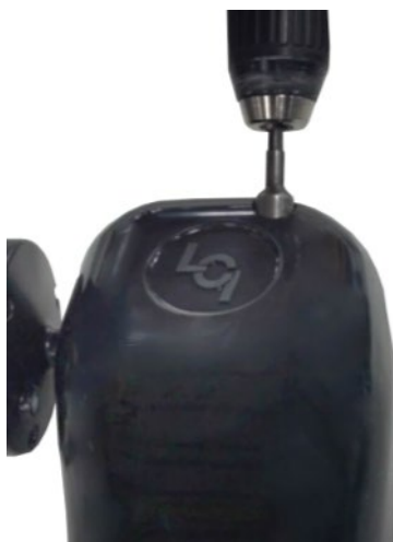
Figure 116. Using a drill to manually retract or extend awning.
