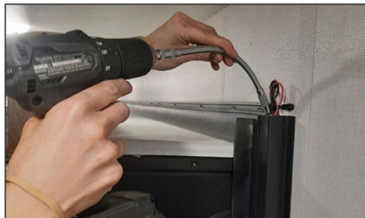
Figure 57. Using the flexible drive tool to manually override the slide.
